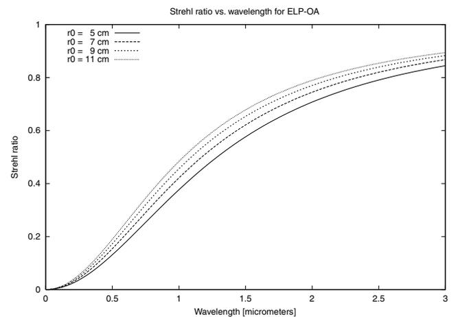
**Figure 5.** Maximum Strehl ratio versus wavelength for values of  $r_0$  ranging from 5 to 11 cm for the original configuration denoted ‘ELP-OA III’ in Table 1. Optimal integration times range from 12 ms ( $r_0 = 5$  cm) to 19 ms ( $r_0 = 11$  cm).
