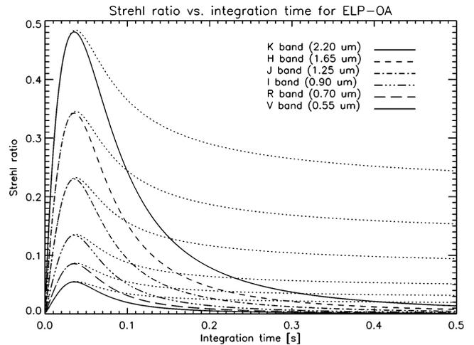
**Figure 4.** Strehl ratio versus integration time for several astronomical observation bands for the configuration denoted ‘ELP-OA II’ in Table 1 and  $r_0 = 10$  cm. Solid and dashed lines, high-bandwidth approximation; dotted lines, exact solution. The optimal integration time,  $t_{i,\text{max}}$ , is 35 ms.
