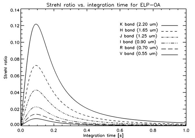
**Figure 2.** Strehl ratio versus integration time for several astronomical observation bands for the original configuration of ELP-OA (‘ELP-OA I’ in Table 1) and  $r_0 = 10$  cm (at 0.5  $\mu\text{m}$ ). The high-bandwidth approximation was used to calculate these results. The optimal integration time,  $t_{i,\text{max}}$ , is 92 ms.
