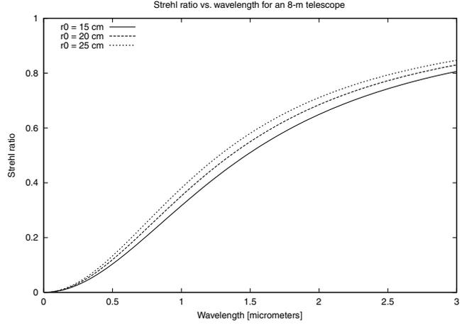
**Figure 6.** Maximum Strehl ratio versus wavelength for values of  $r_0$  ranging from 15 to 25 cm for the 8-m configuration denoted ‘8-m I’ in Table 1. Optimal integration times range from 42 ms ( $r_0 = 15$  cm) to 56 ms ( $r_0 = 25$  cm).
