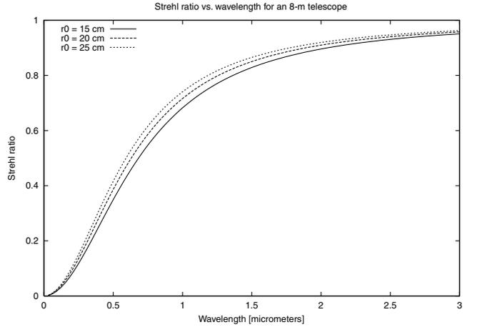
**Figure 7.** Maximum Strehl ratio versus wavelength for values of  $r_0$  ranging from 15 to 25 cm for the 8-m configuration denoted ‘8-m II’ in Table 1. Optimal integration times range from 20 ms ( $r_0 = 15$  cm) to 26 ms ( $r_0 = 25$  cm).
