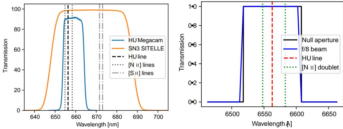
Figure 2: Left: the foreseen filter has similar specifications as the MegaCam  $H\alpha$  filter and is about four times narrower than the current SN3 SITELLE filter. Right: beam aperture blueshifts and broadens filter transmission. Rest-frame wavelengths of the main emission lines are shown as vertical lines.
