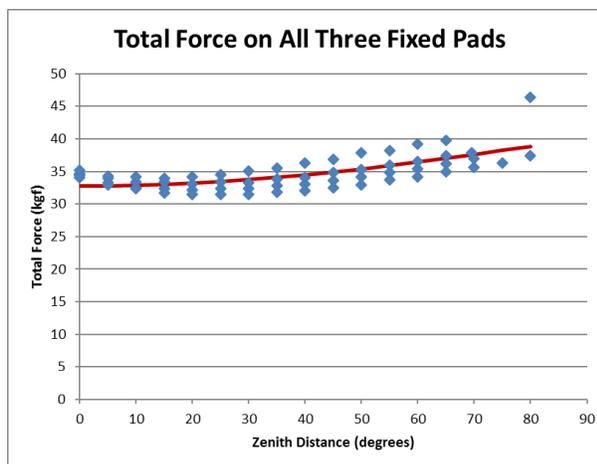
Figure 12 – The summed force over all three fixed pads of the f/8 secondary support system at various telescope angles. The different branches in the data are for telescope motions to the North, South, East and West. The solid line is the predicted force based on fits of the pressure and vacuum data to cosine curves.
