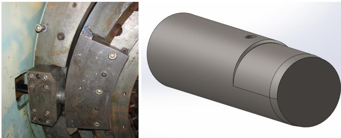
Figure 15 – Declination pin insertion mechanism (left) & new declination pin with relief to provide angular alignment (right).
