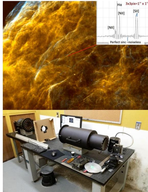
Figure 8 – Top: Emission line spectra from an observing run in March 2016 show both excellent image quality and exquisite FTS instrument line profiles. Bottom: Collimator and camera optics installed on a lab bench for testing off the instrument.
