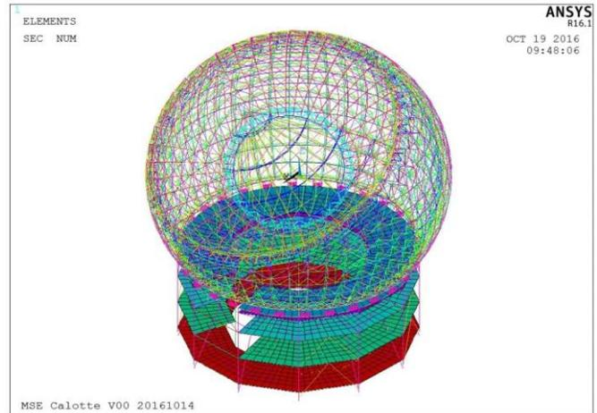
Figure 18 - EDS Calotte FE model.
