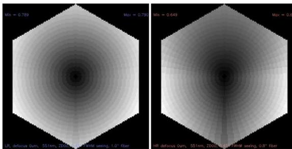
Figure 19 - Grey-scale maps of the injection efficiency as seen by the LMR spectrograph (left) and HR spectrograph (right), at the optimal position, across the entire field of view, with the telescope pointing at zenith, at 551nm, without defocus, with a seeing of 0.45" FWHM, and fibers of 1.0" diameter.
