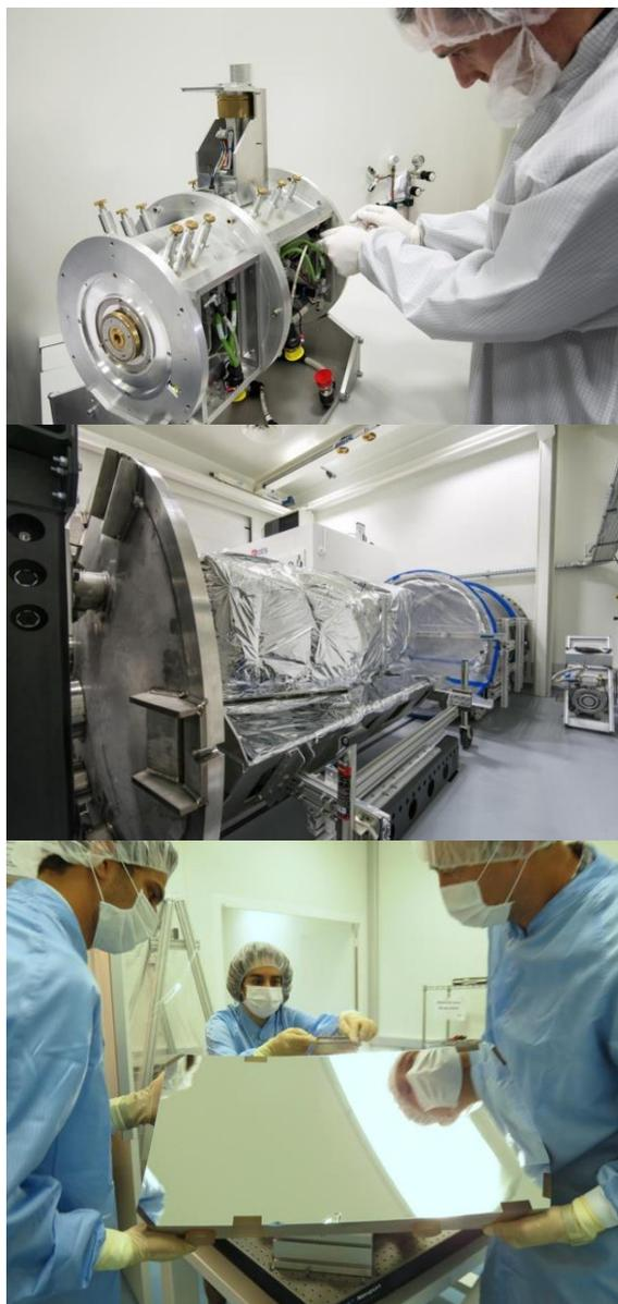
Figure 9 – Top: The Cassegrain feed for SPIRou is shown in the lab at IRAP. Middle: The cryo-bench ready to be enclosed in SPIRou's large vacuum jacket is shown. Bottom: Mounting the parabolic mirror used in double pass in the spectrometer optical assembly is shown.
