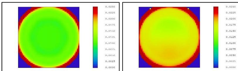
Figure 16 - RMS image quality maps for (left)  $ZD=0^\circ$  and (right)  $ZD=50^\circ$ . The asymmetry in the  $ZD=50^\circ$  case is due to the ADC action.
